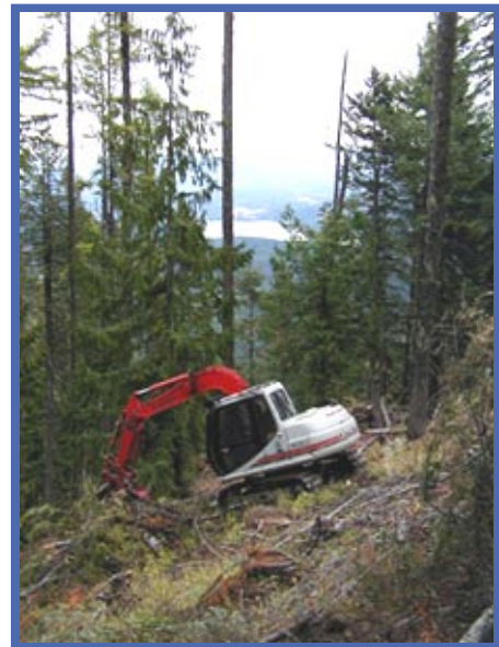
Machine piling logging slash and hazardous fuels.
