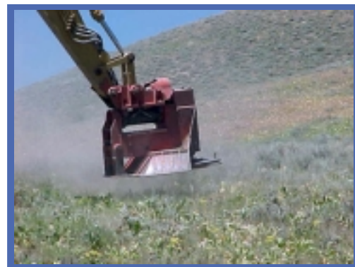
The unique design allows a 270 degree cutting radius for sage and other fuels at a six inch height.
