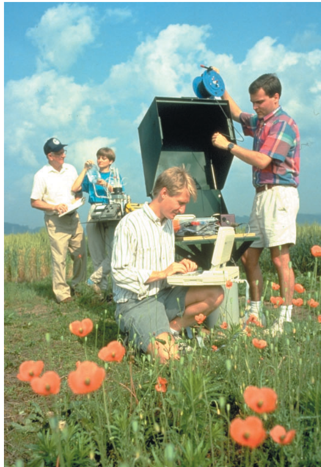
Photo 5-3. As part of USDA's water quality program, ARS and cooperating researchers are investigating the effects of farm pesticides and nitrogen from fertilizer on groundwater. At an Ohio site government researchers and Ohio State University graduate students measure the pH, conductivity, temperature and level of water in a conventional well. (Scott Bauer photo)
