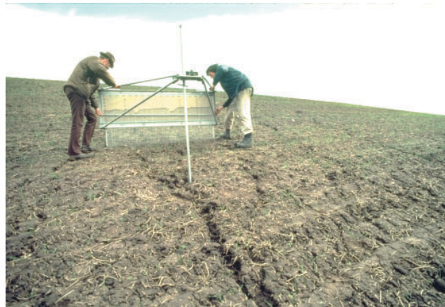
Photo 5-2. Agricultural Research Service (ARS) scientists near Pullman, Washington plot a hillside area where erosion has occurred to gather information for developing better erosion prediction models. (ARS photo)
