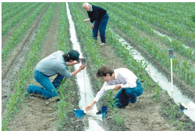
Photo 6-4. USDA technicians in Colorado conduct irrigation delivery tests to determine optimum flow rates and delivery times to improve onfarm irrigation management systems. (Tim McCabe photo)
