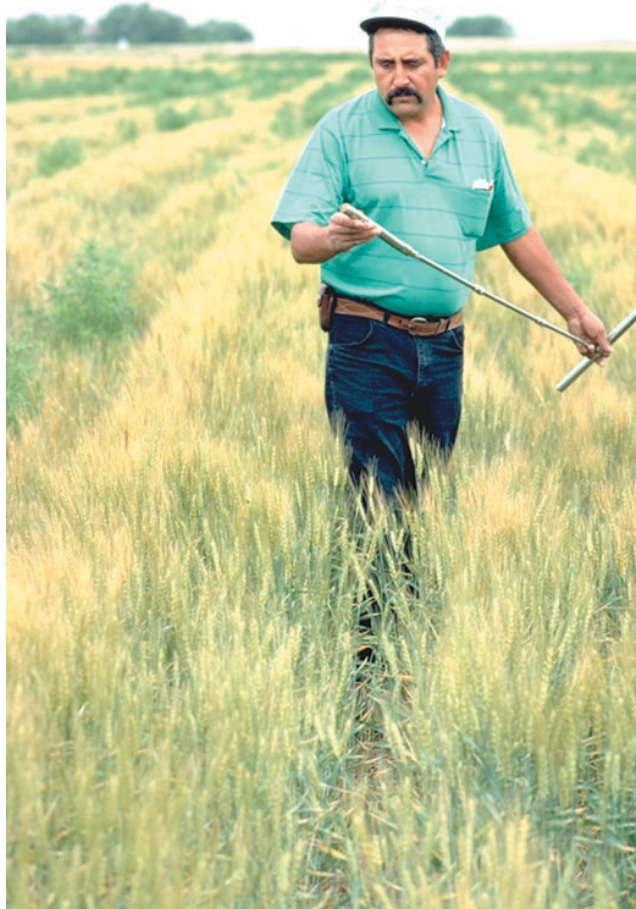
Photo 1-1. A USDA soil specialist uses a probe to sample cropland soils for identification and mapping in the Western United States. (Tim McCabe photo)
