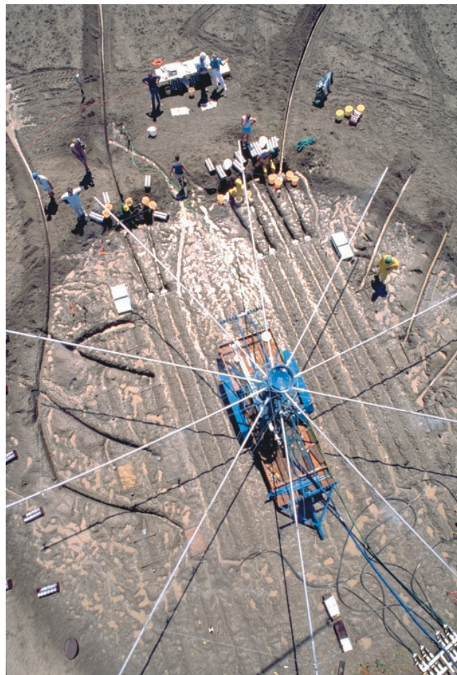
Photo 10-1. Near Cottonwood, SD, scientists from the Agricultural Research Service use a rainfall simulator to gather runoff data on range soils. Data from many range and cropland sites throughout the United States is being used in the development of the WEPP model. (Tim McCabe photo)
