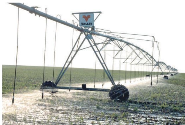
Photo 6-5. LEPA (Low Energy Precision Application) irrigation systems conserve water by keeping delivery low to the ground which greatly reduces drift. Additionally, they offer a variety of nozzle configurations to meet diverse delivery needs. (Tim McCabe photo)
