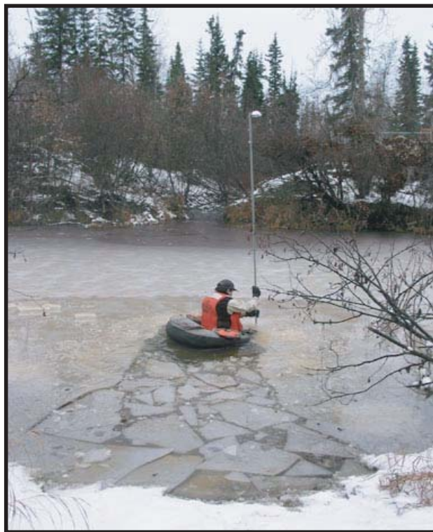
Figure 14. Sampling of streambed sediments under ice cover in Noyes Slough, Fairbanks, Alaska, October 2002.
