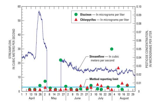
Figure 8. Streamflow, and diazinon and chlorpyrifos concentrations, for the San Joaquin River near Crows Landing, California, sampling site for 2001.
