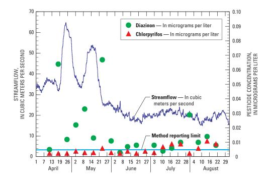
Figure 9. Streamflow, and diazinon and chlorpyrifos concentrations, for the San Joaquin River at Patterson Bridge near Patterson, California, sampling site for 2001.
