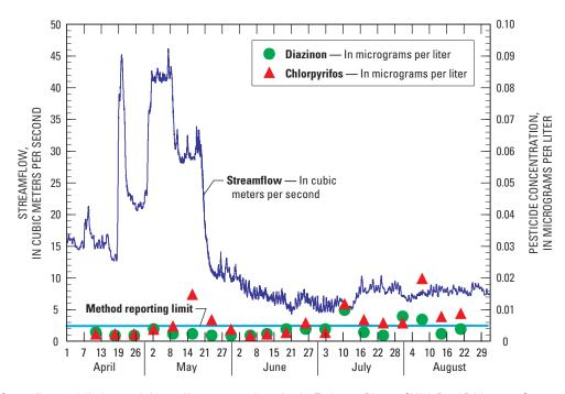
Figure 11. Streamflow, and diazinon and chlorpyrifos concentrations, for the Tuolumne River at Shiloh Road Bridge near Grayson, California, sampling site for 2001.
