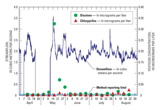
Figure 5. Streamflow, and diazinon and chlorpyrifos concentrations, for the Mud Slough near Gustine, California, sampling site for 2001.
