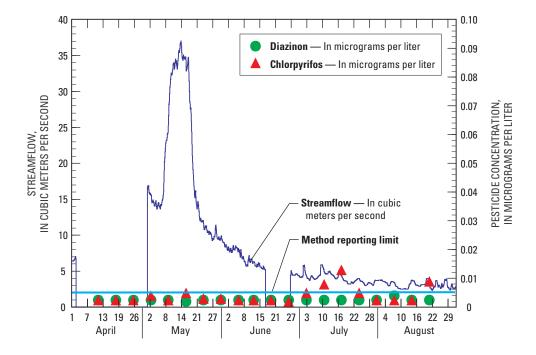
Figure 6. Streamflow, and diazinon and chlorpyrifos concentrations, for the Merced River at River Road Bridge near Newman, California, sampling site for 2001.
