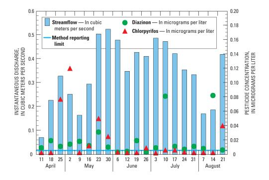
Figure 10. Streamflow, and diazinon and chlorpyrifos concentrations, for the Del Puerto Creek at Vineyard Road near Patterson, California, sampling site for 2001.
