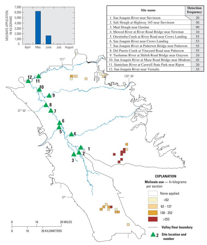
Figure 24. Use of molinate during April through August 2001, and molinate detection frequency at selected sites, San Joaquin Valley, California.
