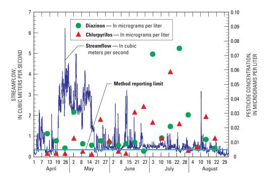
Figure 7. Streamflow, and diazinon and chlorpyrifos concentrations, for the Orestimba Creek at River Road near Crows Landing, California, sampling site for 2001.
