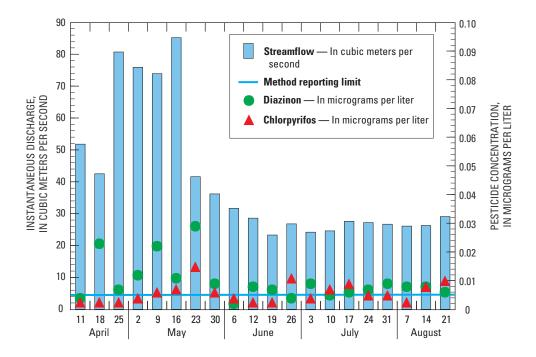
Figure 12. Streamflow, and diazinon and chlorpyrifos concentrations, for the San Joaquin River at Maze Road Bridge near Modesto, California, sampling site for 2001.
