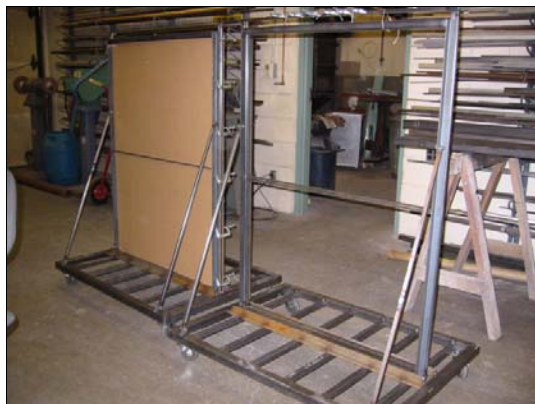
Figure 1. Soil flumes prior to filling with soil.
