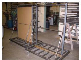
Figure 1. Soil flumes for frozen ground study
