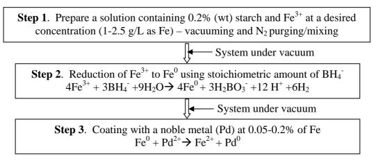
Unlike conventional methods, we applied a low-cost and environmentally friendly carbohydrate (starch) in the preparation. The starch serves as a stabilizer that prevents subsequently formed nanoparticles from agglomeration, thereby maintaining their high
