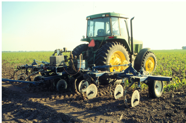
Figure 2. Variable rate anhydrous ammonia toolbar used
