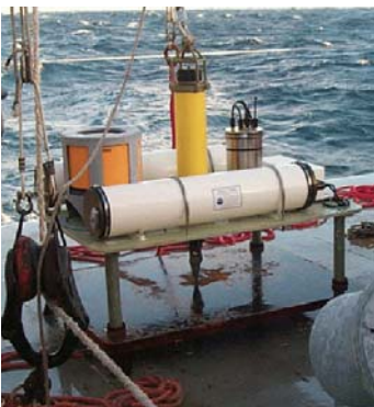
"Tsunami meter" tsunami detection instrumentation
