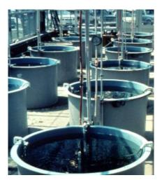
**Fig. 2.** Wild-celery and shoalgrass mesocosms receiving enhanced atmospheric concentrations of carbon dioxide.
