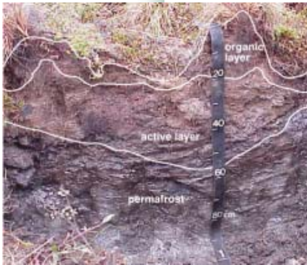
Figure 2b: A soil pit in tussock tundra showing the organic layer, active layer and the permafrost underlying them.
