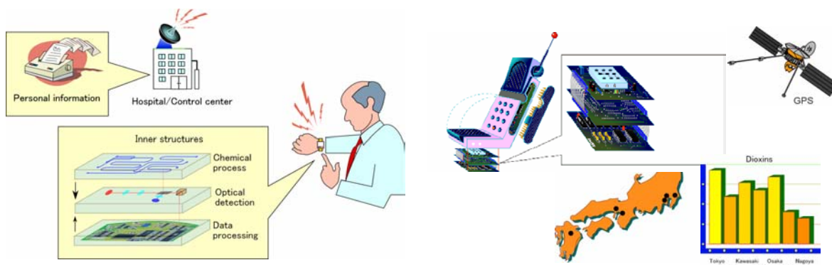
Fig. C.7. Two concepts of integrated chip sensor systems coupled with telemetry methods for remote sensing. Left , a portable ultrasensitive diagnostic device, and, right , an ultratrace pollutant monitoring device.
