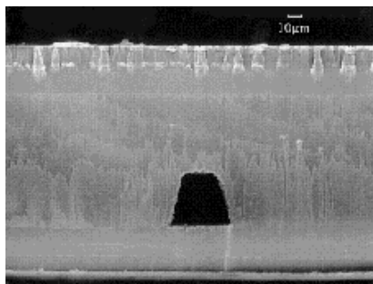
Fig. B.5. SEM view of a cross section of photoablated PET nanospray outlet used for MS analysis (channel dimension: 40 \times 40 \mu\text{m}^2 ).
