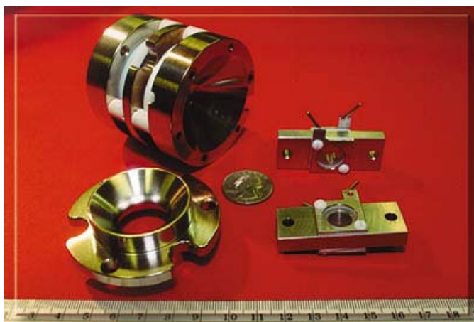
Fig. 5.1. A miniaturized cylindrical ion trap (right) with a commercial ion trap (left) for comparison. (Henry 1999, reprinted with permission)
