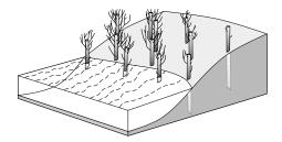
Plantings of cottonwood, willow, poplar, or other species embedded vertically into streambanks to increase channel roughness, reduce flow velocities near the slope face, and trap sediment.
