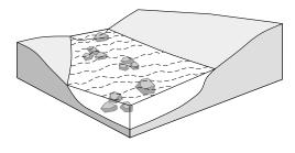
Groups of boulders placed in the base flow channel to provide cover, create scour holes, or areas of reduced velocity.
