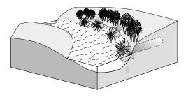
Boulders and logs with root masses attached placed in and on streambanks to provide streambank erosion, trap sediment, and improve habitat diversity.
