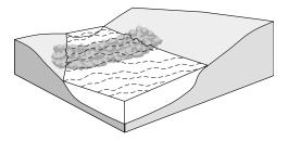
Rock, wood, earth, and other material structures placed across the channel and anchored in the streambanks to provide a "hard point" in the streambed that resists the erosion forces of the degradational zone, and/or to reduce the upstream energy slope to prevent bed scour.
