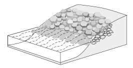
A blanket of appropriately sized stones extending from the toe of slope to a height needed for long term durability.
