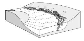
A row of interconnected trees attached to the toe of the streambank or to deadmen in the streambank to reduce flow velocities along eroding streambanks, trap sediment, and provide a substrate for plant establishment and erosion control.
