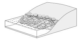
A ridge of quarried rock or stream cobble placed at the toe of the streambank as an armor to deflect flow from the bank, stabilize the slope and promote sediment deposition.
