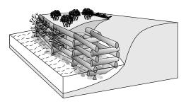
Hollow, box-like interlocking arrangements of untreated log or timber members filled above baseflow with alternate layers of soil material and live branch cuttings that root and gradually take over the structural functions of the wood members.
