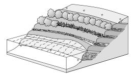
Alternating layers of live branch cuttings and compacted soil with natural or synthetic geotextile materials wrapped around each soil lift to rebuild and vegetate eroded streambanks.
