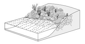
Live stakes tamped into joints or openings between rock which have previously been installed on a slope or while rock is being placed on the slope face.
