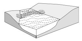
Log, boulder, or quarrystone structures placed across the channel and anchored to the streambank and/or bed to create pool habitat, control bed erosion, or collect and retain gravel.
