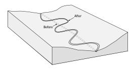
Transformation of a straightened stream into a meandering one to reintroduce natural dynamics improve channel stability, habitat quality, aesthetics, and other stream corridor functions or values.
