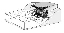
Wire-mesh, rectangular baskets filled with small to medium size rock and soil and laced together to form a structural toe or sidewall. Live branch cuttings are placed on each consecutive layer between the rock filled baskets to take root, consolidate the structure, and bind it to the slope.
