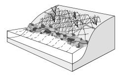
Combination of live stakes, live facines, and branch cuttings installed to cover and physically protect streambanks; eventually to sprout and establish numerous individual plants.
