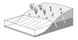
Live, woody cuttings which are tamped into the soil to root, grow and create a living root mat that stabilizes the soil by reinforcing and binding soil particles together, and by extracting excess soil moisture.
