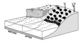
Regrading streambanks to a stable slope, placing topsoil and other materials needed for sustaining plant growth, and selecting, installing and establishing appropriate plant species.
