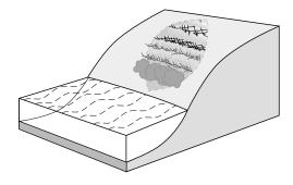
Alternate layers of live branches and compacted backfill which stabilize and revegetate slumps and holes in streambanks.
