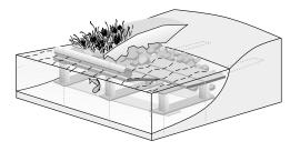
Cells constructed of heavy wooden planks and blocks which are imbedded into the toe of streambanks at channel bed level to provide covered compartments for fish shelter, habitat, and prevention of streambank erosion.
