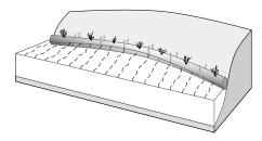
Cylindrical structures composed of coconut husk fibers bound together with twine woven from coconut material to protect slopes from erosion while trapping sediment which encourages plant growth within the fiber roll.
