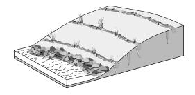
Dormant branch cuttings bound together into long sausage-like, cylindrical bundles and placed in shallow trenches on slopes to reduce erosion and shallow sliding.
