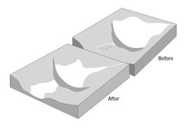
A high-magnitude, short duration release from a reservoir to scour fine-grained sediments from the streambed and restore suitable instream habitat.
