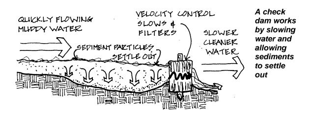
Types of velocity controls and energy dissipaters include:
