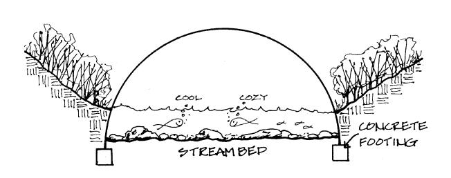
Bottomless arch culvert to accommodate fish passage
