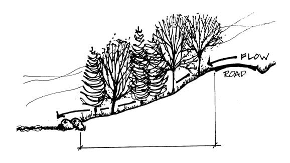
Cross section of a filter zone
