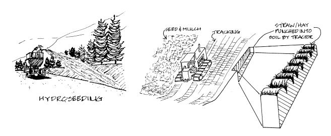
Hydroseeding and surface roughening, two low cost ways to stabilize a slope
