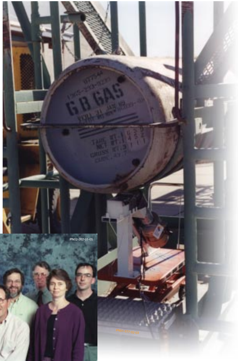
The PINS technology was adapted to detect small quantities of mercury at the bottom of large nerve gas containers (top and right). The team includes from left to right (front row) Bob Gehrke (ret.), Gus Caffrey and Ann Egger; (back row) Steve Frickey, Ken Krebs, Larry Blackwood, Andy Edwards and Ed Seabury. Not pictured are John Zabriskie, John Baker and Cathy Riddle.
