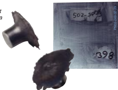
A marksman zeros in a rifle to test a new ceramic armor composite; a hydraulic dolly used to raise the armor sample into position for ricochet tests; an actual armor sample and the resultant flattened slugs from a successful armor test.
