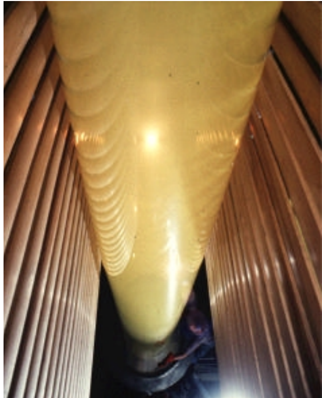
A towering stable bubble of polymer film. New polymer architectures and realistic modeling will allow extremely rapid manufacturing of these films that avoid the bubble dance.
