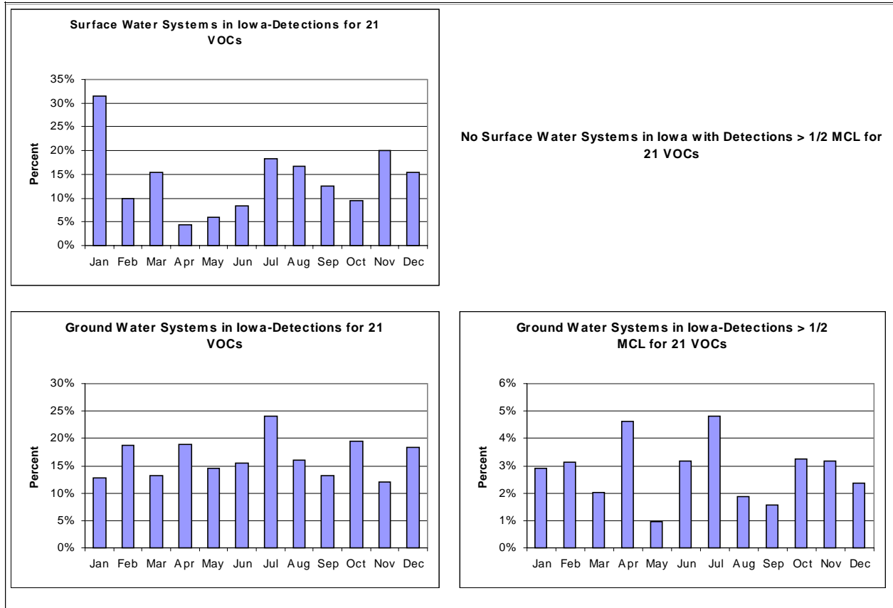
Figure V.C.8. Percentage of systems with detections (>MRL, >0.5MCL) of any of the 21 regulated VOCs, by month, for Iowa.
