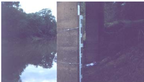
Staff gages similar to this one will be installed near several bridges in the NWS Norman HSA. Photo courtesy of Daryl Williams, Hydrometeorological Technician.
