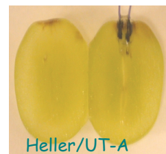
Figure 7. A biofuel cell that operates using the glucose fuel and water innate to a grape.
