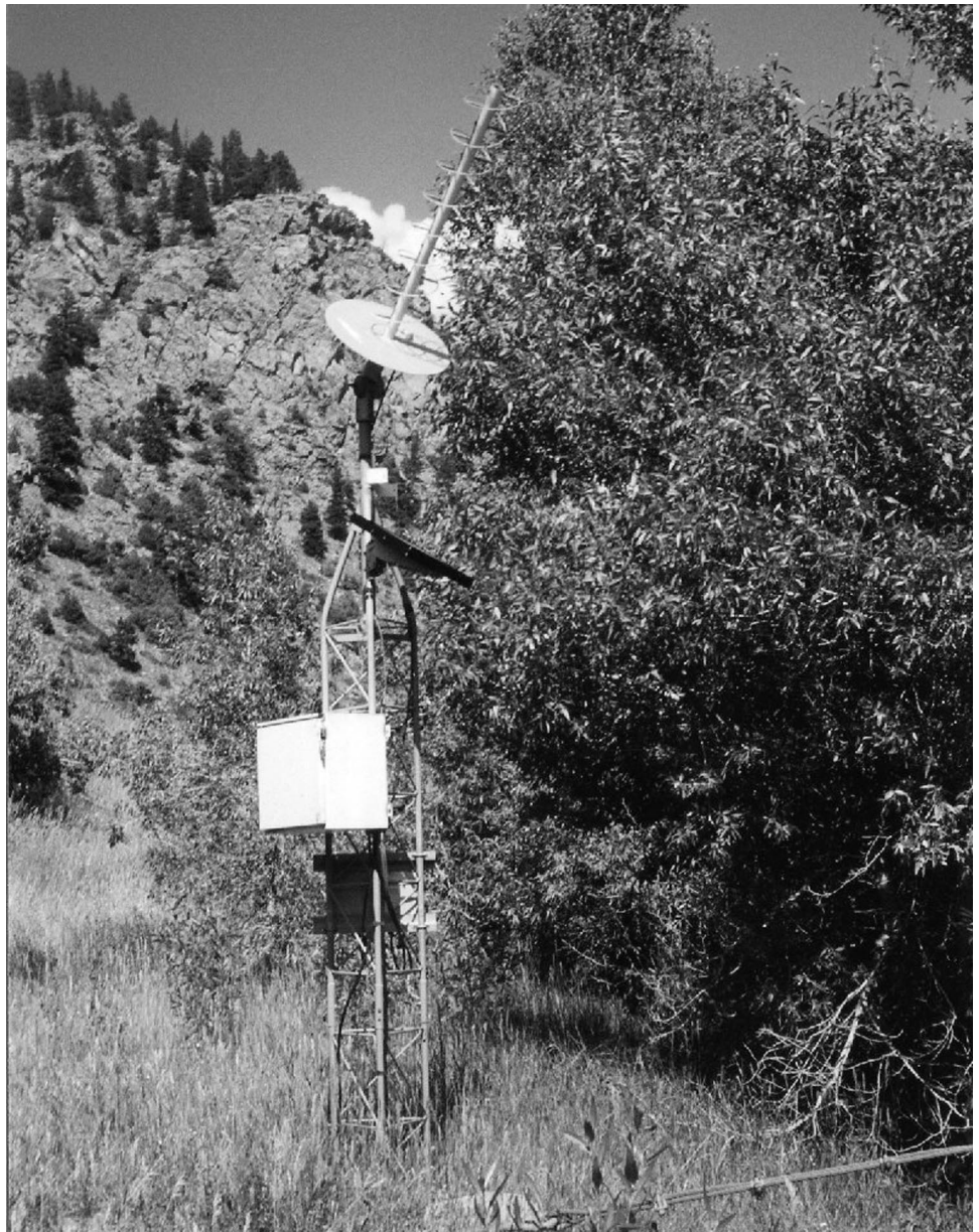
Figure 11: Satellite Used to Relay Collected Water Quantity Data to Data Users (Lawson, Colorado)
