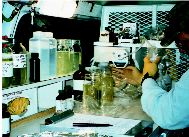
Water samples are filtered and processed in a mobile laboratory immediately after sample collection.
