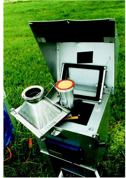
The yellow polyurethane foam plug was used to collect pesticides distributed into the gas phase of the atmosphere.
