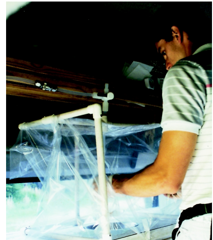
Ground-water sample preparation occurred inside plastic enclosures in order to minimize sample contamination from chemicals in the atmosphere.
