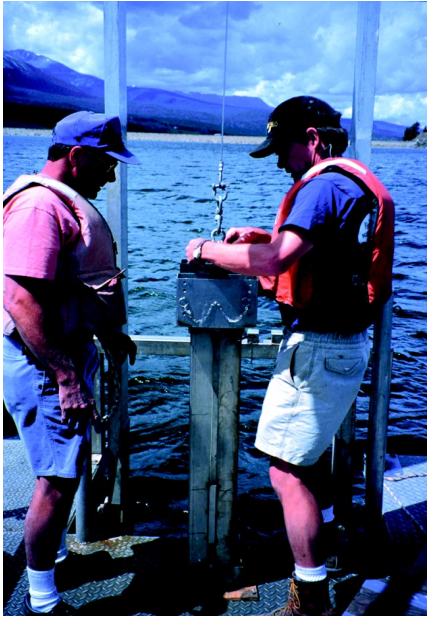
Collecting sediment core samples on Dillon Reservoir. (Photograph by Norman Spahr, U.S. Geological Survey.)
