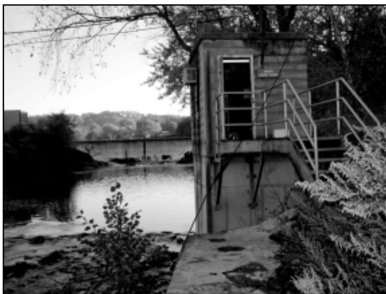
Figure 1. Flow-through water-quality monitoring station. (PHOTOGRAPH: RAMAPO RIVER AT POMPTON LAKES, NEW JERSEY, BY MICHAEL J. DELUCA)
