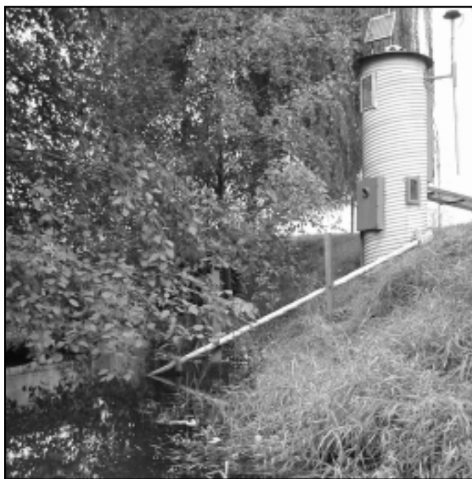
Figure 2. In-situ water-quality monitoring station. (PHOTOGRAPH: SPRING BROOK CREEK AT ORILLIA, WASHINGTON, BY DAVID K. MULLIS)
