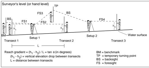
Figure 6. Diagram of how to measure water-surface gradient with a clinometer or surveyor's level.
