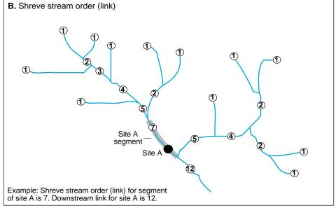
**Figure 3.** Examples of how to calculate (A) Strahler stream order and (B) Shreve stream order (link) and downstream link.
