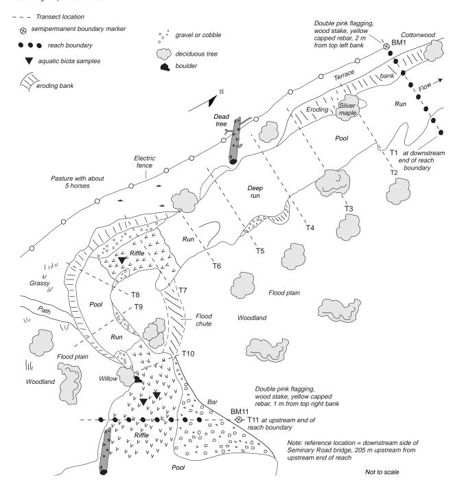
**Figure 5.** Example of a diagrammatic stream map showing transect locations, reach boundary markers, and other important stream characteristics.
