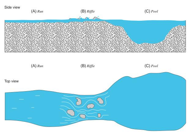
**Figure 4.** Diagram of the three main geomorphic channel units. (A) Run—A slow moving, relatively shallow body of water with moderately low velocities and little or no surface turbulence; (B) Riffle—A part of the stream where the water flows swiftly over completely or partially submerged obstructions to produce surface agitation; (C) Pool—A part of the stream with reduced velocity, commonly with deeper water than surrounding areas (modified from Bisson and others, 1982).
