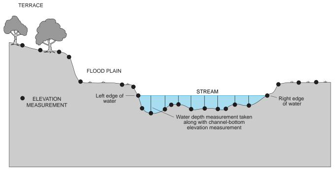
Figure 13. Example of measurement points for cross-section profiles.
