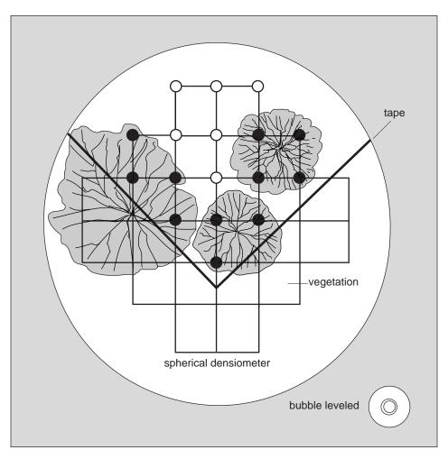
**Figure 10.** A concave spherical densiometer with bubble level, tape, and 17 points of observation. Line of intersections at both open and closed circles are examined. Closed circles represent line intersections counted in measurement of canopy closure (11 out of 17 points).
