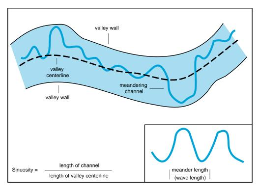
Figure 2. Example of how to measure sinuosity.
