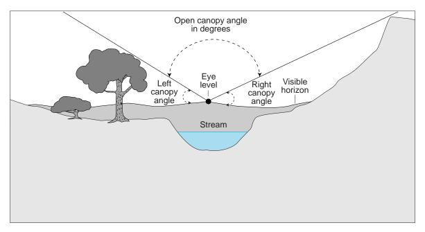
Figure 9. Measurement of open canopy angle (modified from Platts and others, 1983).
