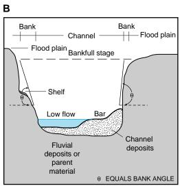
**Figure 7.** Examples of the relative position of geomorphic features, bankfull stage, and bank angle from (A) a bend in a meandering stream, and (B) a straight reach.
