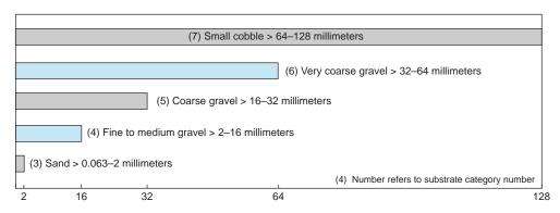
Figure 11. Field scale for identifying particle-size classes from sand to small cobble.
