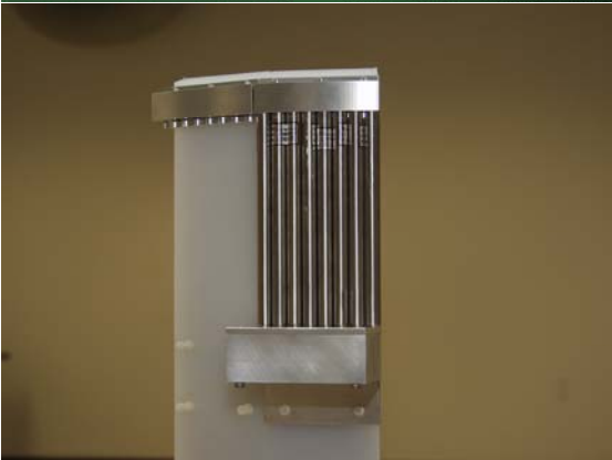
First production detectors for the Backscattering Spectrometer mounted in the prototype rig
