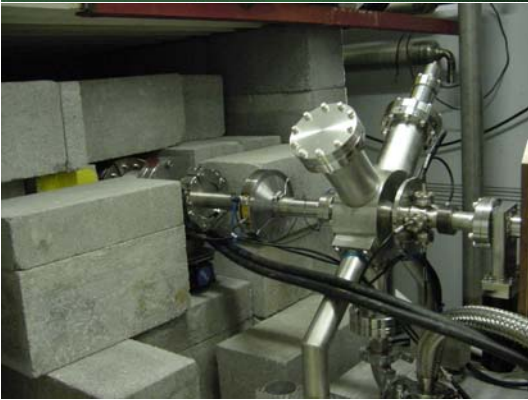
CCL-2 Beam Stop installed in the Linac Tunnel
