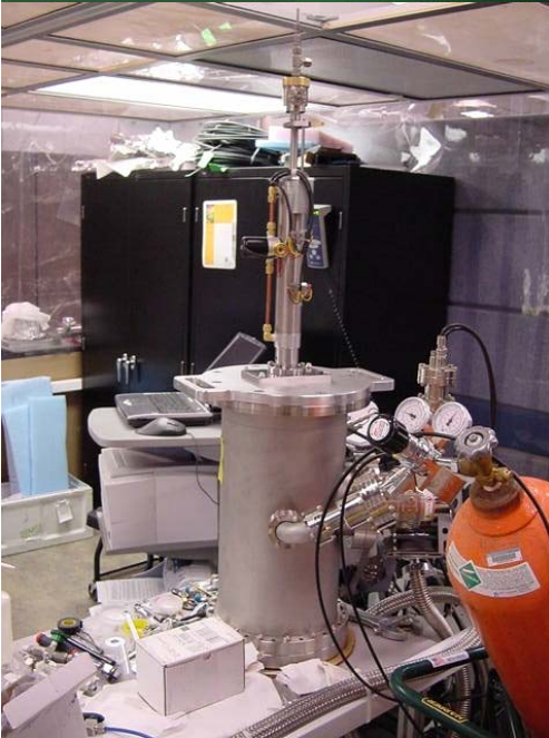
DTL Vacuum Test Stand at ORNL
