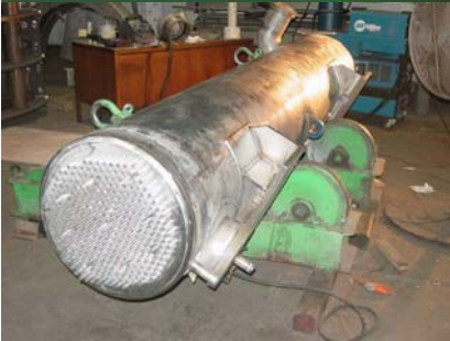
Fabrication of the Mercury Water Heat Exchanger
