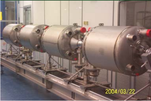
String assembly for cryomodule High-β 1
