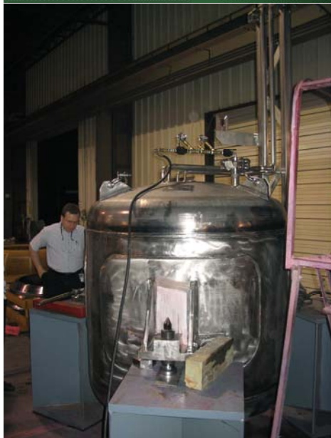
Mercury Storage Tank
